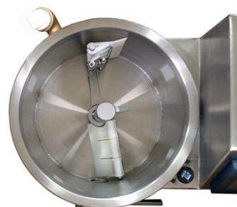
Removable agitator with bottom and sidewall scraping action
