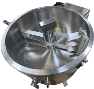
Removable agitator with bottom and sidewall scraping action
